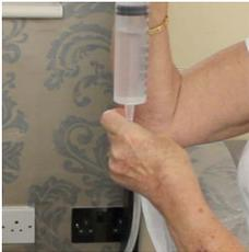
3. Insert syringe into open end of U-drain tubing and plunge solution into the system.
